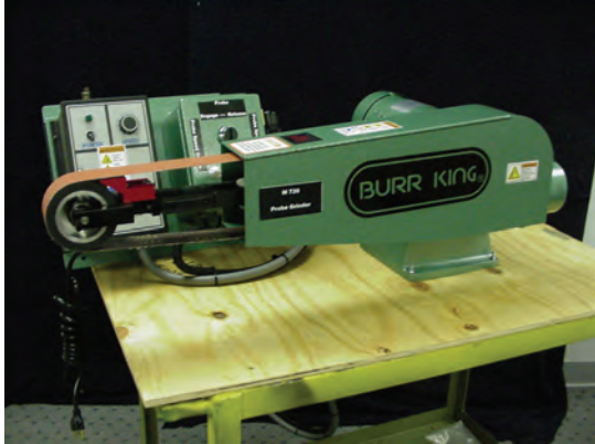
Picture 1: Shown, a model 720 with optional 4 inch diameter wheel, variable speed, with remote control console. Note guard door is closed and latched.
