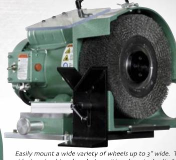
Easily mount a wide variety of wheels up to 3" wide. The side door is a hingeless design with only a single clip for access to the wheel.
